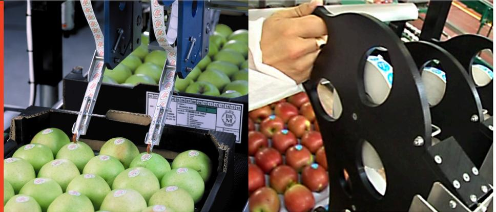
The **BCS** is a machine especially made for fresh produce labeling in 50 x 30 cm and 60 x 40 cm trays. The tray passes, narrow edge leading under the labeling head. This is the easiest and most economic system.
