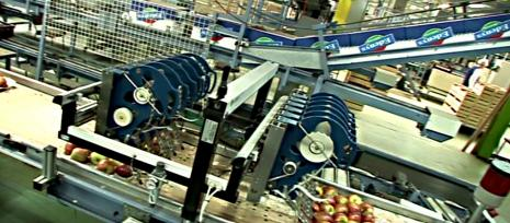
he BCA is a multi-purpose system made for fresh produce labeling in trays and inners. The frame can be made in the same way as for the BCS, that is to say a metallic frame to be directly mounted on the conveyor. As an extra option, the customer may also get the aluminium frame with a mechanized height adjustment.
